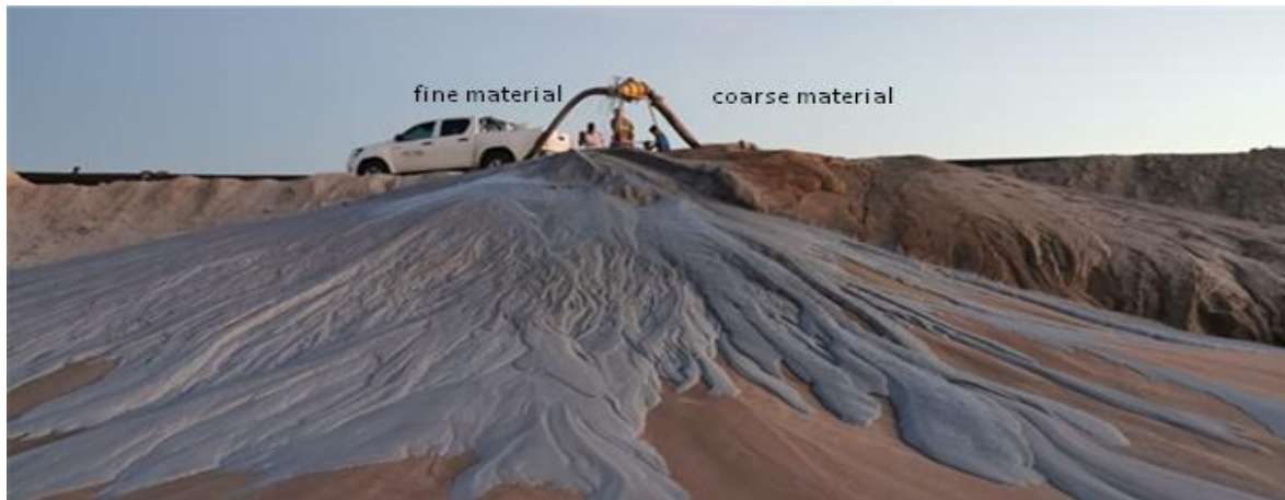
Figure 14: Example of cyclone deposition
