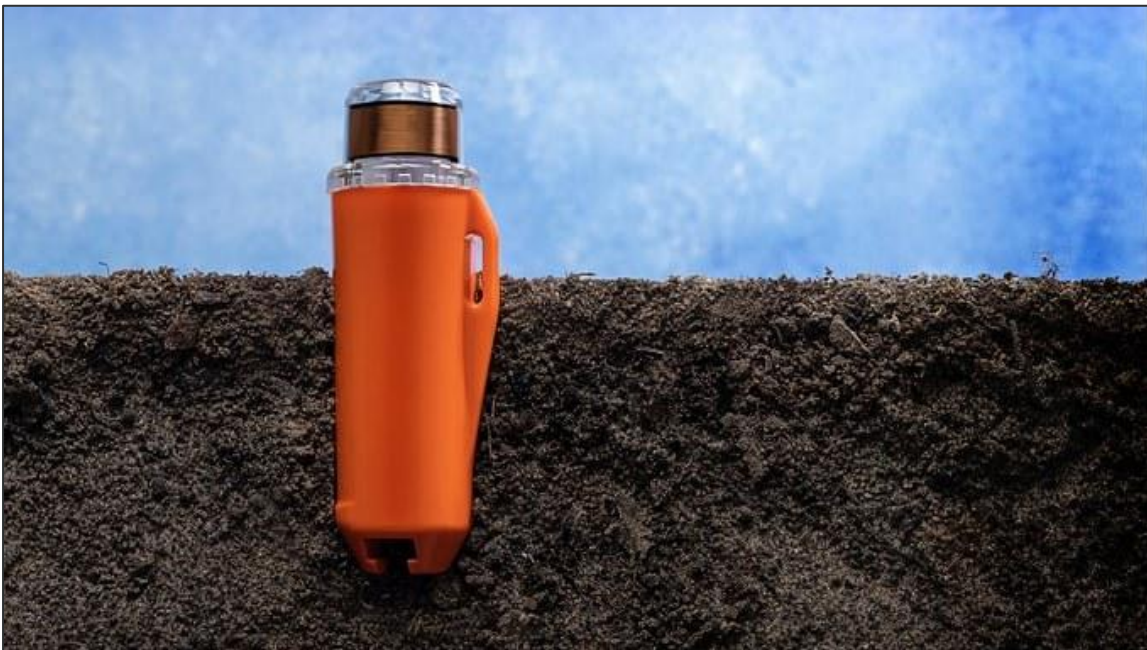
Figure 4: A STRYDE's Node™. Wireless nodal system to be used as the land seismic receiver system in conjunction with the Nomad 65 vibroseis trucks (STRYDE, 2022).
