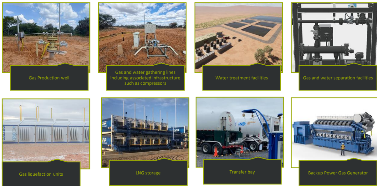
Figure 5: List of surface infrastructure and example pictures.
