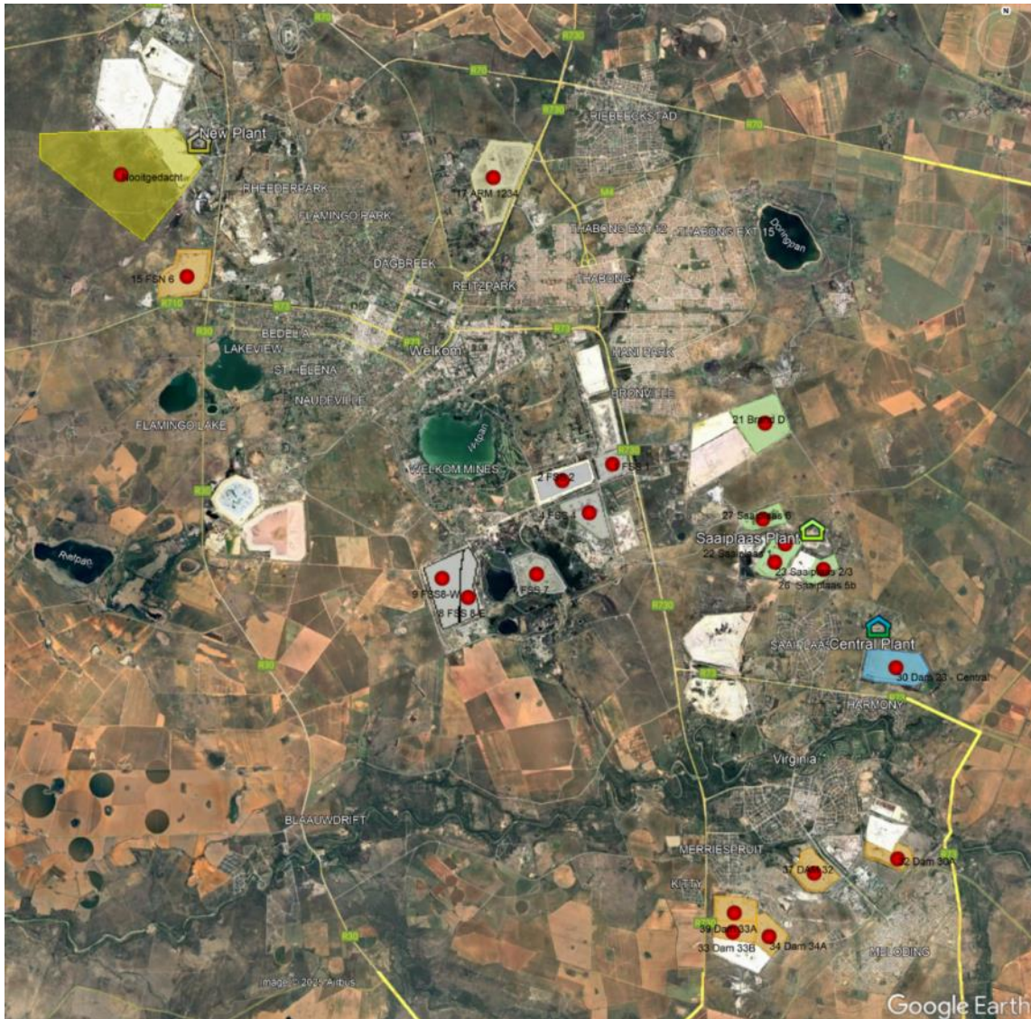
Figure 65: Nineteen existing unlined Tailings Storage Facilities (TSFs) will be reclaimed and deposited onto the new lined Nooitgedacht TSF
