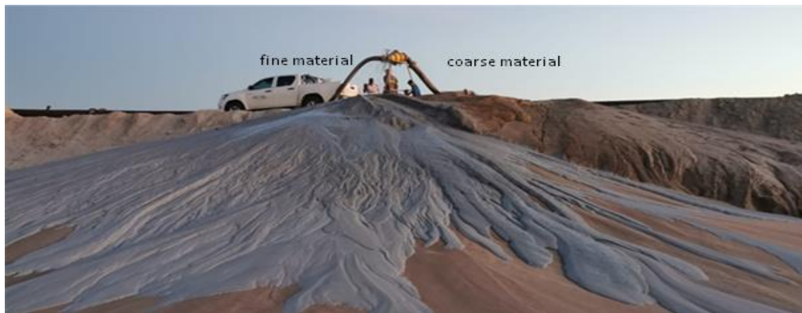
Figure 16: Example of cyclone deposition
