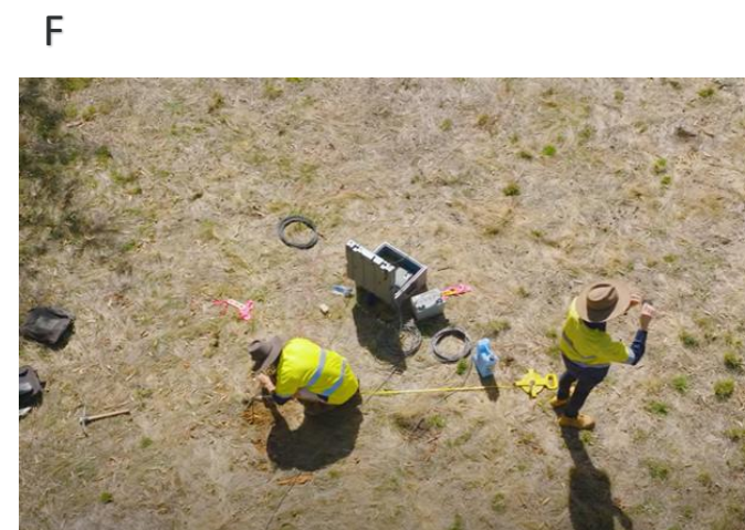
Figure 5: Seismic surveying process and potential impacts. (A) Showing an animated Vibroseis process, (B) Showing a real life Vibroseis process, (C) Showing minimal dust generated from the process, (D) Showing minimal vegetation impact associated with a new access path (transect route), (E) Showing the weight drop alternative method and (F) showing magnetotelluric survey.
