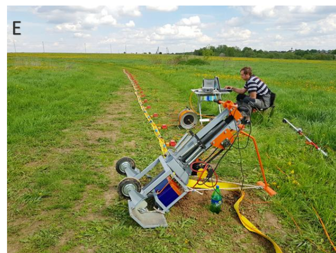
Figure 5: Seismic surveying process and potential impacts. (A) Showing an animated Vibroseis process, (B) Showing a real life Vibroseis process, (C) Showing minimal dust generated from the process, (D) Showing minimal vegetation impact associated with a new access path (transect route), (E) Showing the weight drop alternative method and (F) showing magnetotelluric survey.
