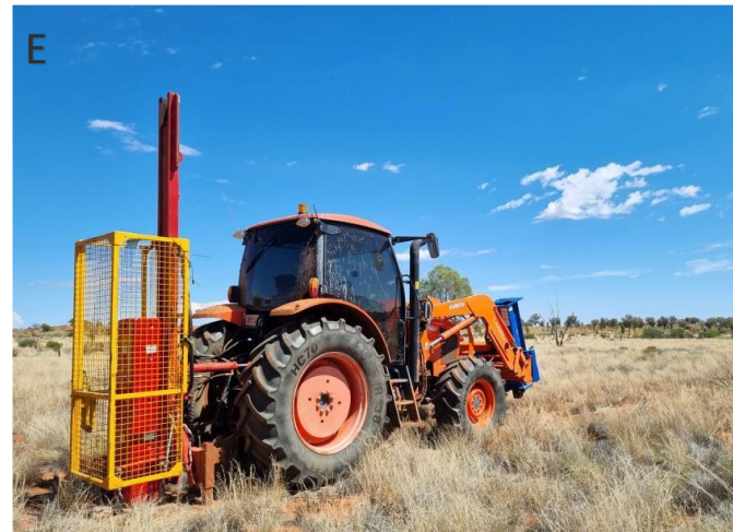
Figure 7: Seismic surveying process and potential impacts. (A) Showing an animated Vibroseis process, (B) Showing a real life Vibroseis process, (C) Showing minimal dust generated from the process, (D) Showing minimal vegetation impact associated with a new access path (transect route), (E) Showing the weight drop alternative method and (F) showing magnetotelluric survey.
