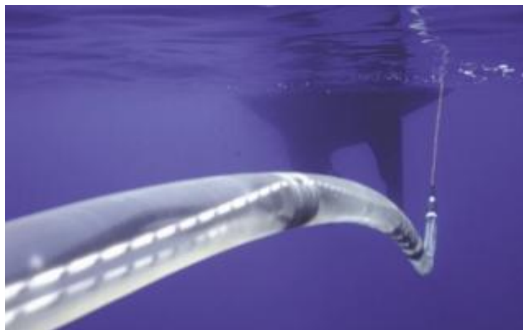
Figure 6: Typical Marine Stream containing hydrophones.
