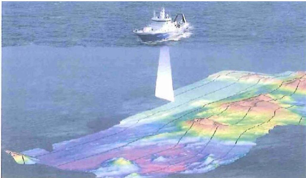
Figure 3.4: Illustration of a vessel using multi-beam depth/echo sounders ( http://www.gns.cri.nz/ ).
