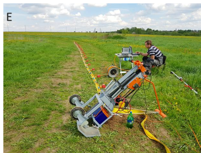
Figure 3: Seismic surveying process and potential impacts. (A) Showing an animated vibroseis process, (B) Showing a real life vibroseis process, (C) Showing minimal dust generated from the process, (D) Showing minimal vegetation impact associated with a new access path (transect route), (E) Showing the weight drop alternative method and (F) showing magnetotelluric survey.
