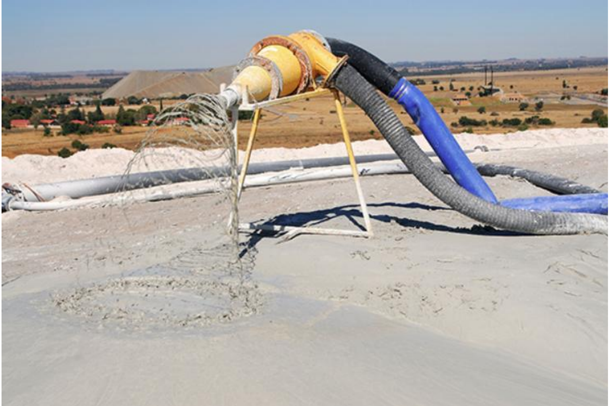
Figure 31: Example of cyclone deposition (Goldfields, 2023)
