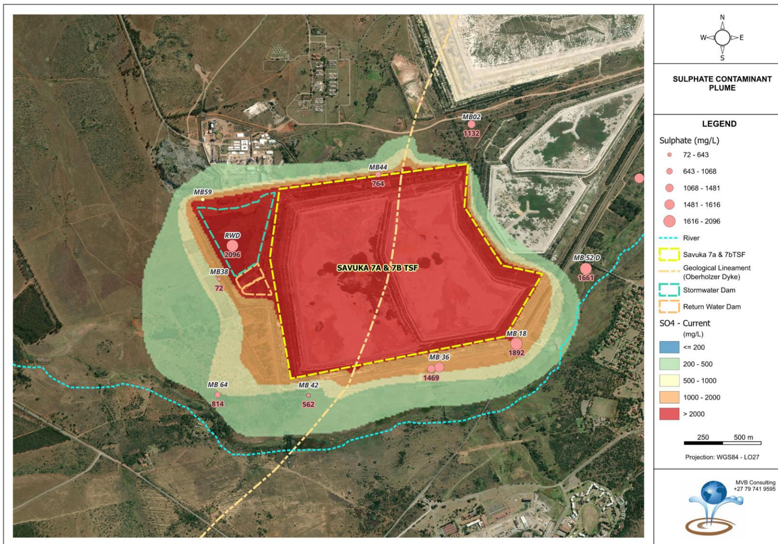
Figure 36: Current simulated plume compared to the measured SO 4 concentrations
