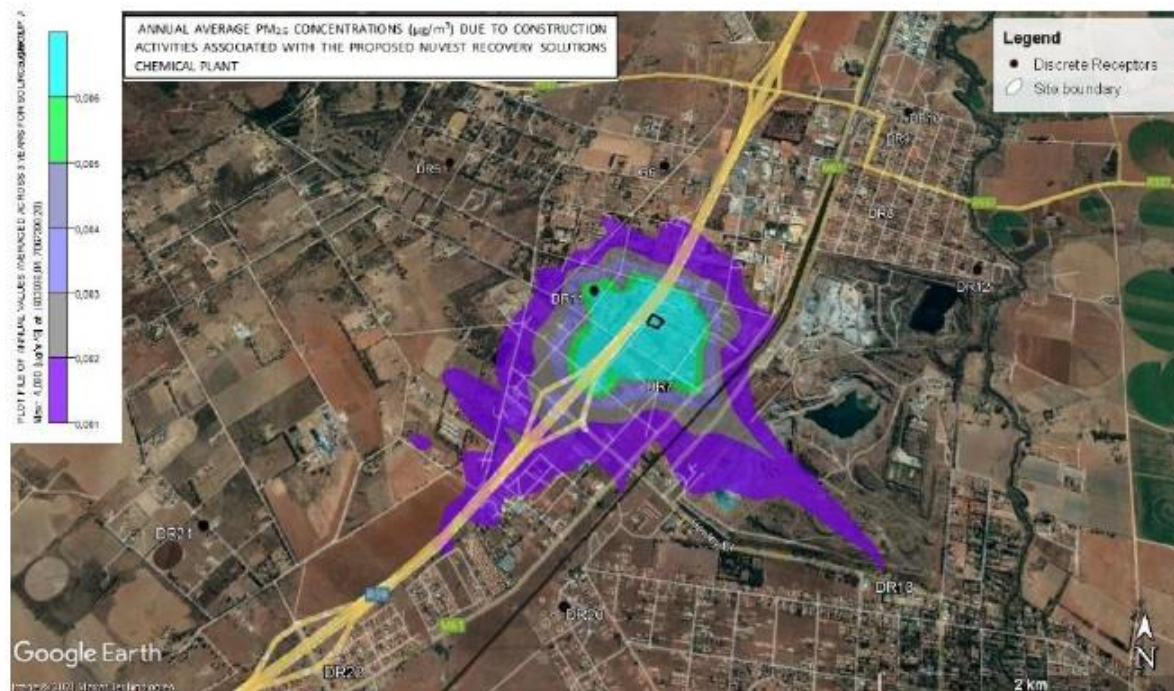
Figure 38: Predicted PM 2.5 annual average incremental concentrations at the project site: Construction Phase (Rayten Engineering Solutions, 2023).
