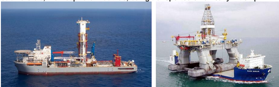
Figure 5.1: Example of a drill rig, the Noble Globetrotter II (left) and of a semi-submersible, the Deepwater Nautilus, being transported on a heavy-lift ship
