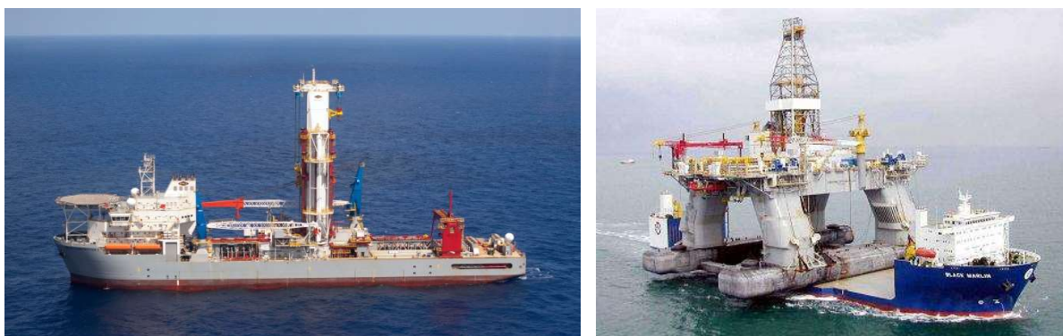
Figure 1.2: Example of a drill rig, the Noble Globetrotter II (left) and of a semi-submersible, the Deepwater Nautilus, being transported on a heavy-lift ship.
