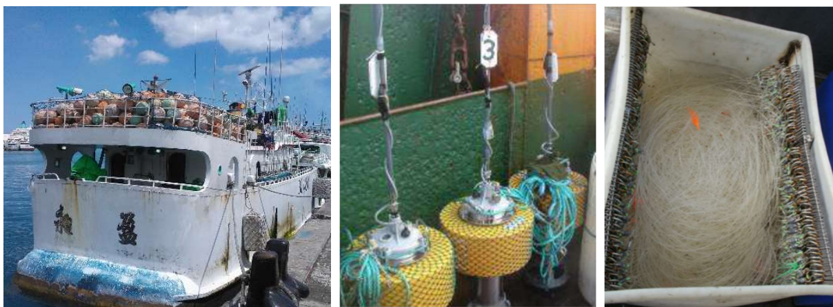
Figure 3.41: Photographs showing marker buoys (left), radio buoys (centre) and monofilament branch lines (right) (Source: CapMarine, 2015).
