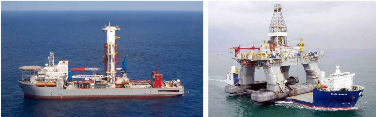
Figure 2: Example of a drill rig, the Noble Globetrotter II (left) and of a semi-submersible, the Deepwater Nautilus, being transported on a heavy-lift ship.
