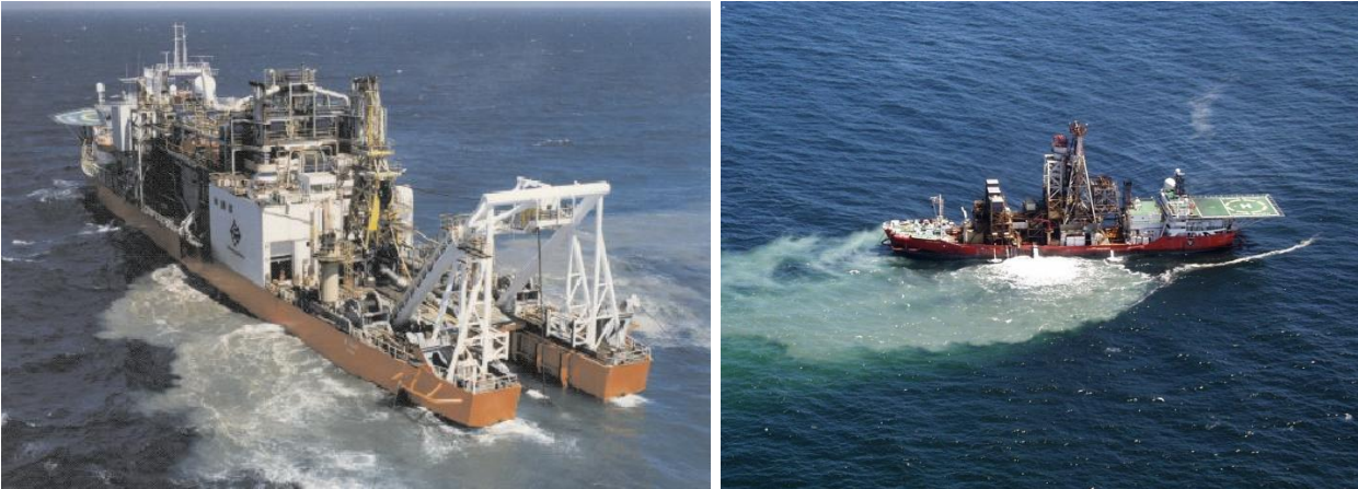
Figure 50: Typical crawler-vessel (left) and drillship (right) operating in the Atlantic 1 Mining Licence Area (Photos: De Beers Marine).
