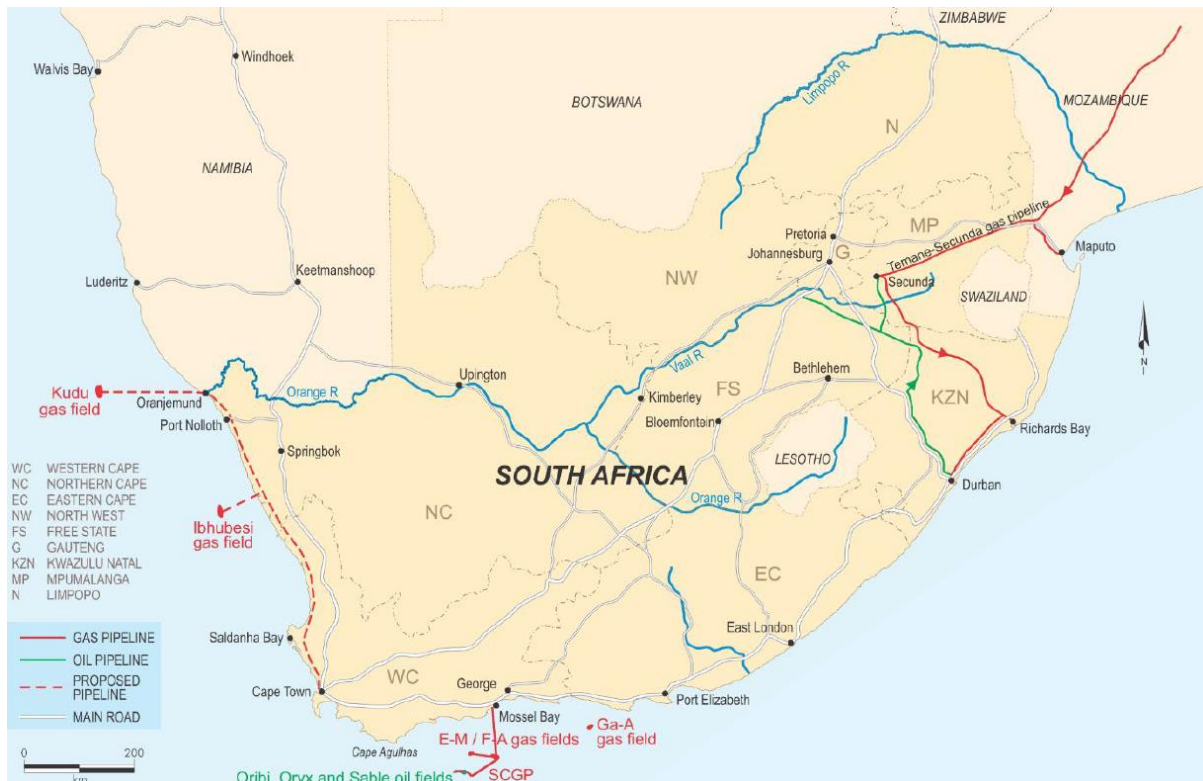
Figure 171: Gas Import and Domestic Production Infrastructure
