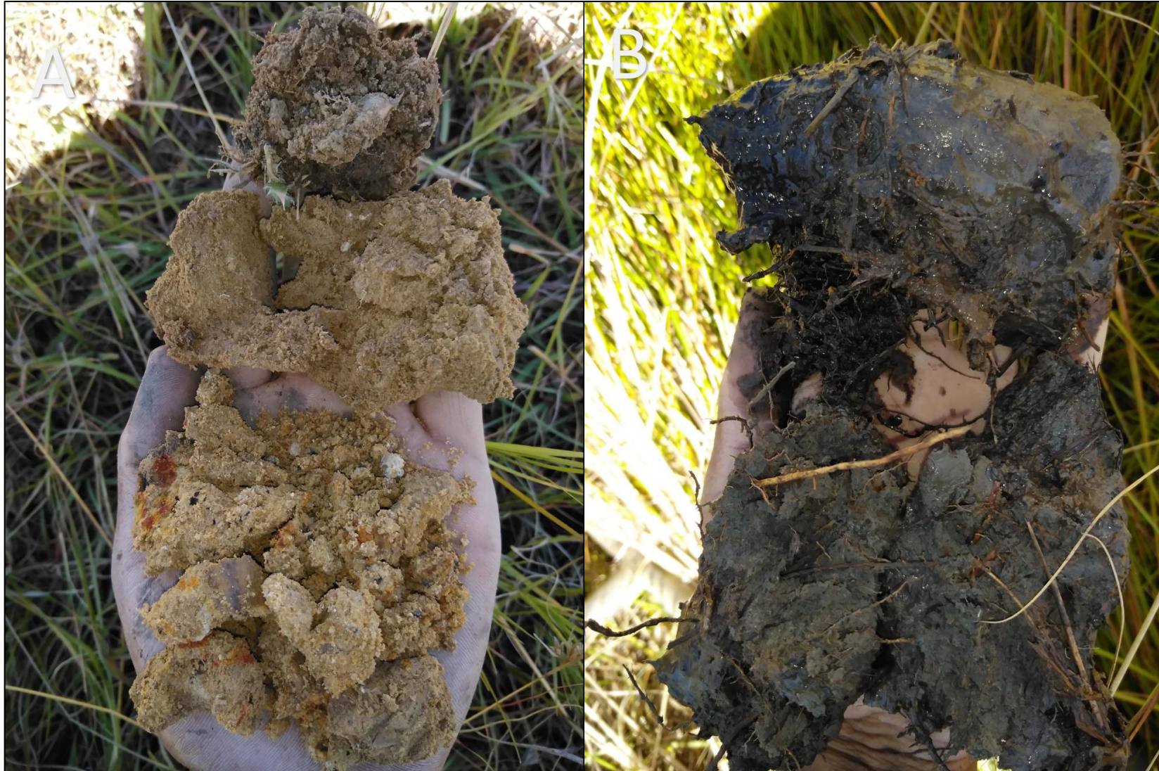
Figure 5-1 Dominant soils identified during the site assessment: A) Orthic topsoil with a Yellow-Brown apedal subsurface horizon. B) Gley horizon below.
