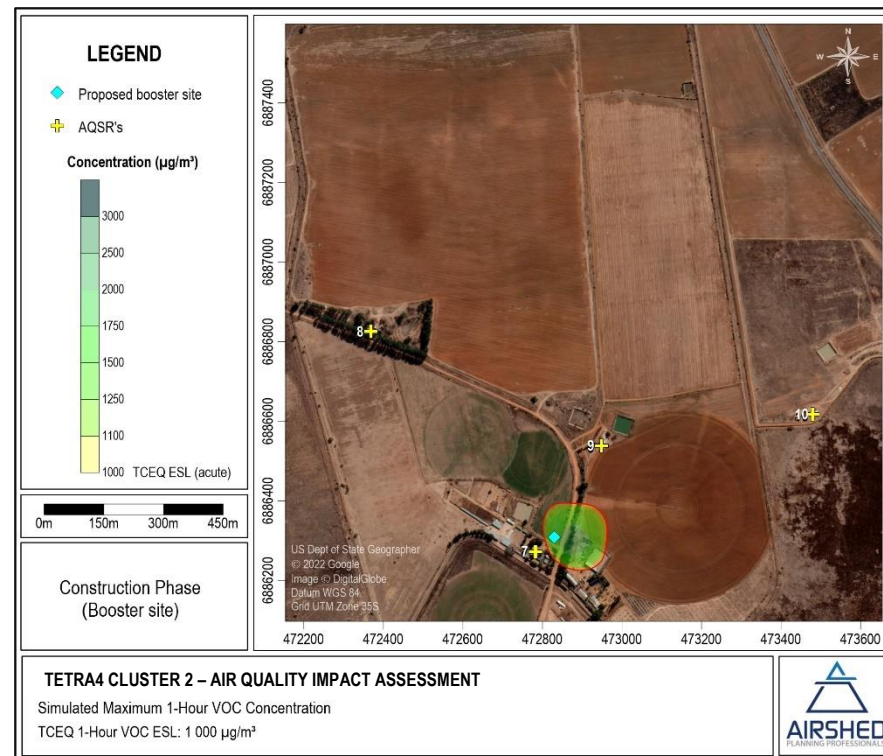
Figure 24: Simulated maximum 1-hour VOC GLCs due to proposed booster station construction emissions (single exceedance of TCEQ ESL up to 130 m beyond booster site indicated as red line)
