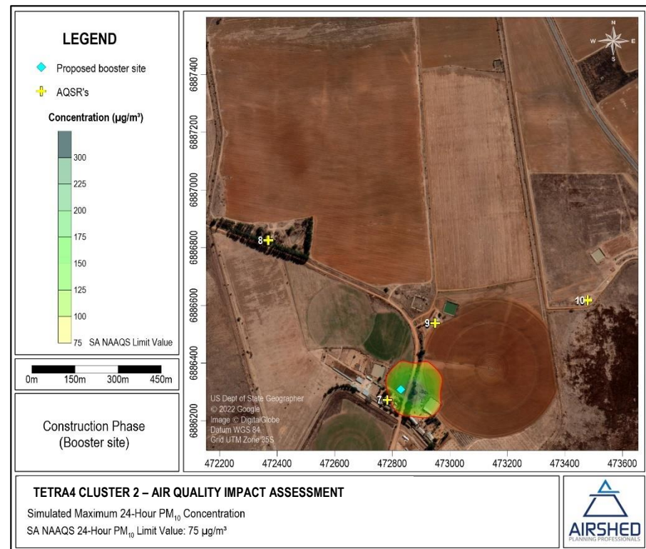
Figure 13: Simulated maximum 24-hour \text{PM}_{10} GLCs due to proposed booster station construction emissions (single exceedance of NAAQS limit up to 150 m beyond booster site indicated as red line)
