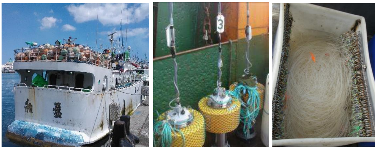
Figure 3.24: Photographs showing marker buoys (left), radio buoys (centre) and monofilament branch lines (right) (Source: CapMarine, 2015).
