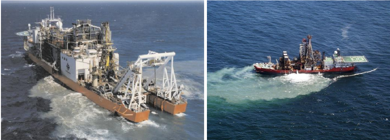
Figure 39: Typical crawler-vessel (left) and drillship (right) operating in the Atlantic 1 Mining Licence Area (Photos: De Beers Marine).
