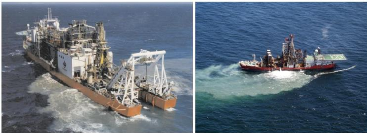
Figure 87: Typical crawler-vessel (left) and drillship (right) operating in the Atlantic 1 Mining Licence Area (Photos: De Beers Marine).
